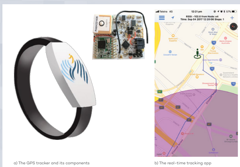
Figure 8. LoRa GPS tracker for dementia wandering monitoring supports.
